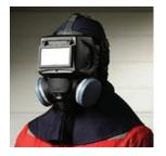
This is a twin-filter respirator with welding visor. It has two P3 filters. The welding visor can be removed to allow the RPE to be worn with suitable PPE for other tasks, eg grinding.
