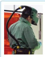
The filter and fan are mounted on the waist belt of this battery powered welding kit. It delivers filtered air to the welder from the flexible hose at the back of the unit.
